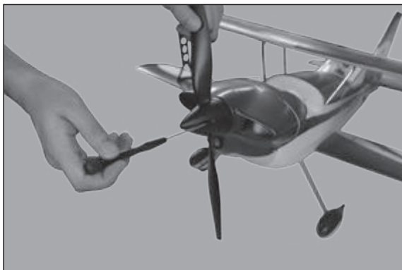
17 Install spinner with PA2.5*8mm screws.
